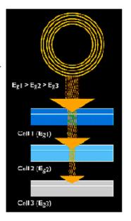
One way to get around this limitation is to use two (or more) different cells, with more than one band gap and more than one junction, to generate a voltage. These are referred to as "multijunction" cells (also called "cascade" or "tandem" cells). Multijunction devices can achieve a higher total conversion efficiency because they can convert more of the energy spectrum of light to electricity.
