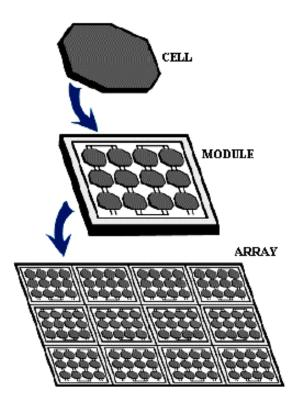
Multiple modules can be wired together to form an array. In general, the larger the area of a module or array, the more electricity that will be produced. Photovoltaic modules and arrays produce direct-current (dc) electricity. They can be connected in both series and parallel electrical arrangements to produce any required voltage and current combination.
