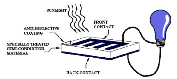
The diagram above illustrates the operation of a basic photovoltaic cell, also called a solar cell. Solar cells are made of the same kinds of semiconductor materials, such as silicon, used in the microelectronics industry. For solar cells, a thin semiconductor wafer is specially treated to form an electric field, positive on one side and negative on the other. When light energy strikes the solar cell, electrons are knocked loose from the atoms in the semiconductor material.
