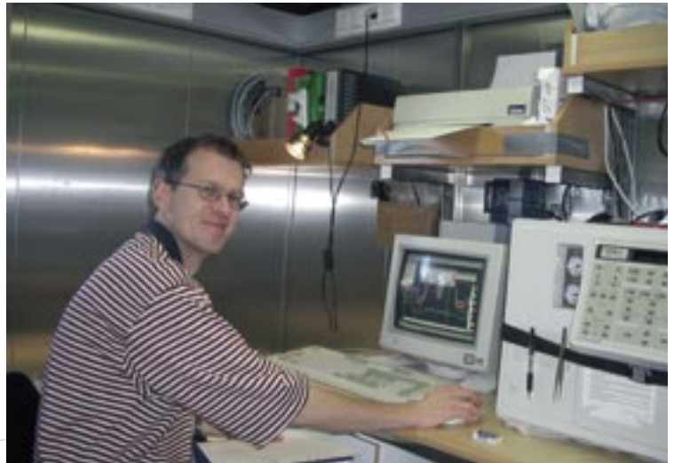
Anders Olsson determines freons in seawater by gaschromatography on board R/V G.O. Sars.
