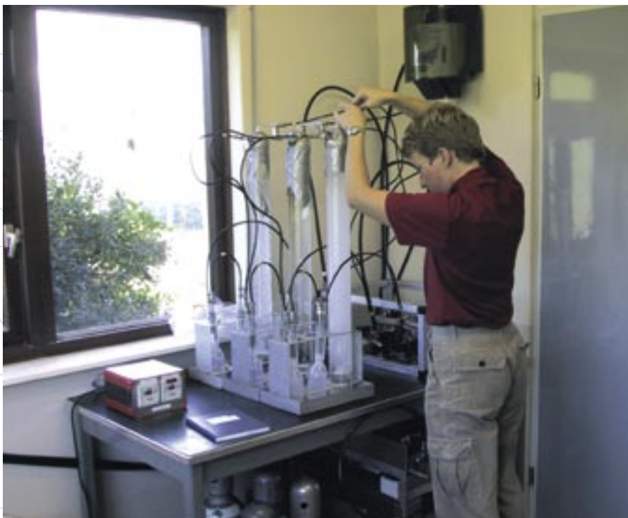
At the atmospheric monitoring station Lutfjewad on the North Sea coast (The Netherlands), biweekly-integrated \text{CO}_2 samples are taken by absorption of \text{CO}_2 in sodium hydroxide for Radiocarbon-analysis.
