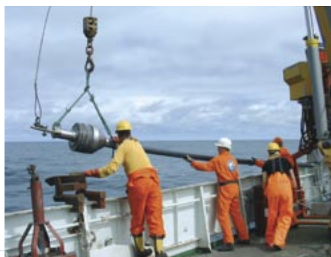
Deployment of gravity corer in the Faroe-Shetland Channel during a NO-Clim cruise on board R/V Håkon Mosby.
