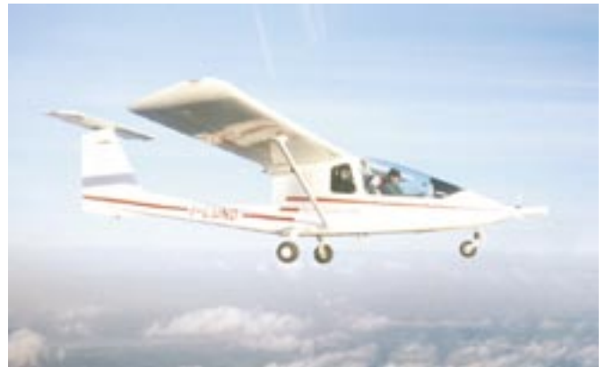
SkyArrow, the world's smallest certified research aircraft, measures the fluxes of CO 2 and water vapour.
